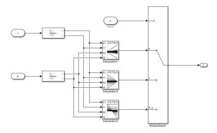
The model contains three Interpolation Using Prelookup blocks that take inputs from the Prelookup1 and Prelookup2 blocks. The outputs of the Interpolation Using Prelookup blocks connect to a Multiport Switch block. This model satisfies the preceding the conditions.
